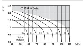
$I_{A}$  = actual ripple current at 120Hz,
