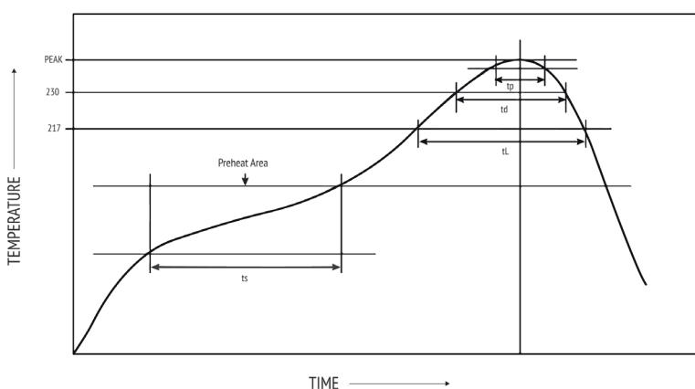
Only 1 reflow soldering cycle allowed. All temperatures are measured on the topside of the Al-can.
