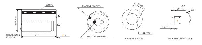
Standard Version: Self-Lock Terminal. Other terminal types and styles on request. For diameter  $øD \ge 45$ mm the safety vent is typically placed at the side of the housing.
