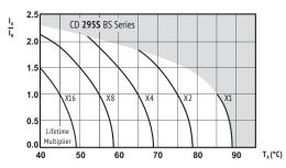
$I_{A}$  = actual ripple current at 120Hz,
