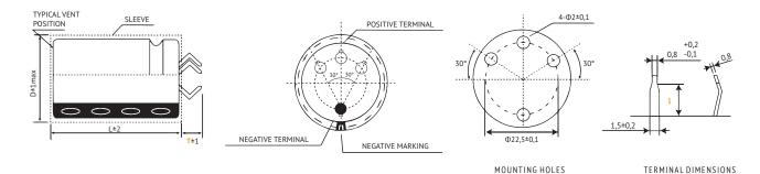
For  $øD \ge 30$ mm only. Other terminal types and styles on request. For diameter  $øD \ge 45$ mm the safety vent is typically placed at the side of the housing.
