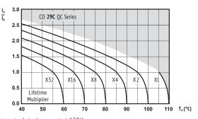
$I_{A}$  = actual ripple current at 120Hz,  $I_{R}$  = rated ripple current at 120Hz, 105°C
