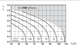
$I_A$  = actual ripple current at 120Hz,
