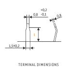
Standard Version: Self-Lock Terminal. Other terminal types and styles on request. For diameter  $\emptyset D \geqslant 45$  mm the safety vent is typically placed at the side of the housing.
