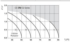
I<sub>A</sub> = actual ripple current at 120Hz,
