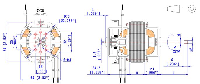
Remarks: Both the rear bracket and front bracket heights or shape can be changeable as needed.
