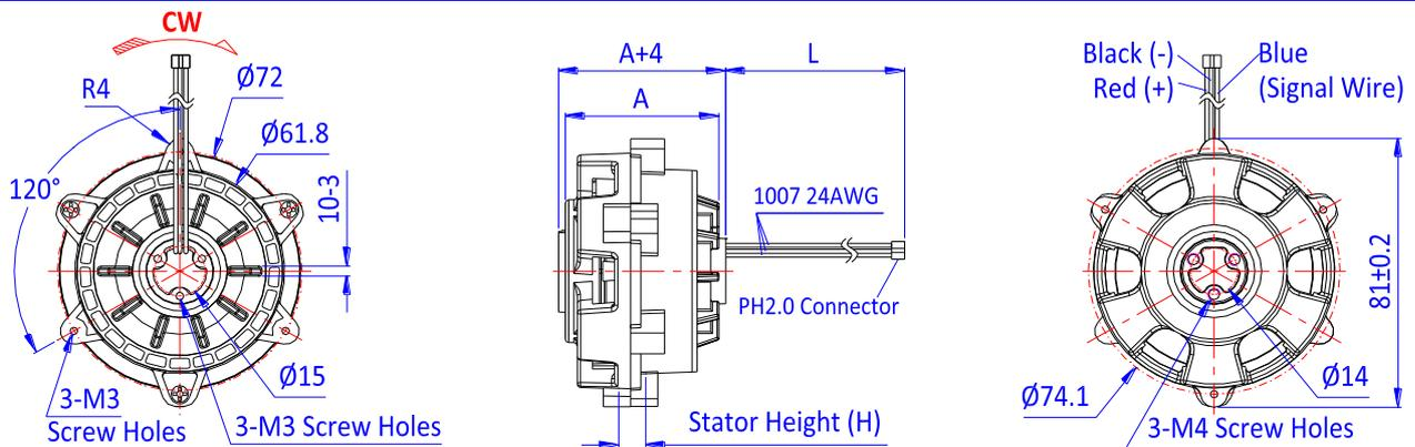
Indication of Letters: A: Motor body length H: Height of stator lamination L: Power cord length
