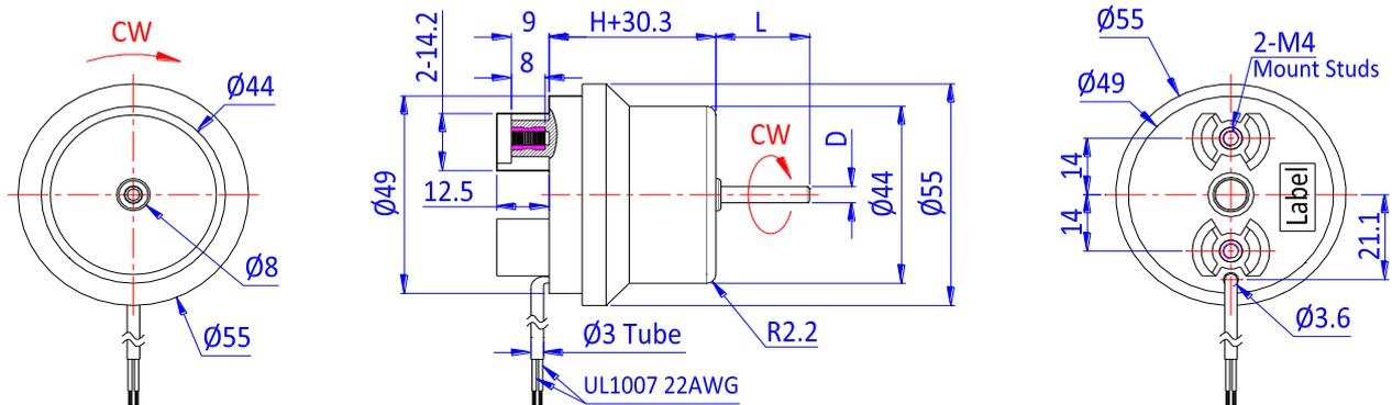
Indication of Letters: D: Shaft Diameter L: Shaft Extended Length H: Stator Lamination Height
