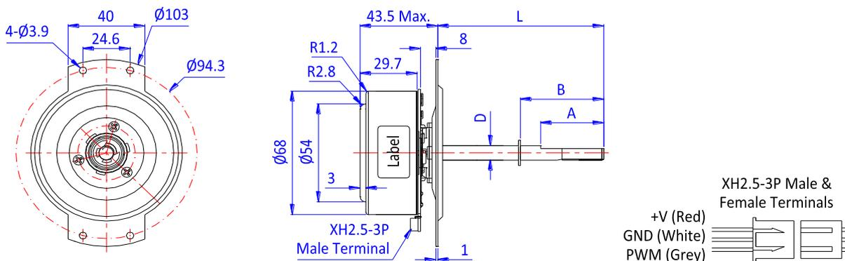
Indication of Letters: D: Shaft Diameter L: Shaft Extended Length A: D-cut Length B: Length from shaft end to the snap ring
