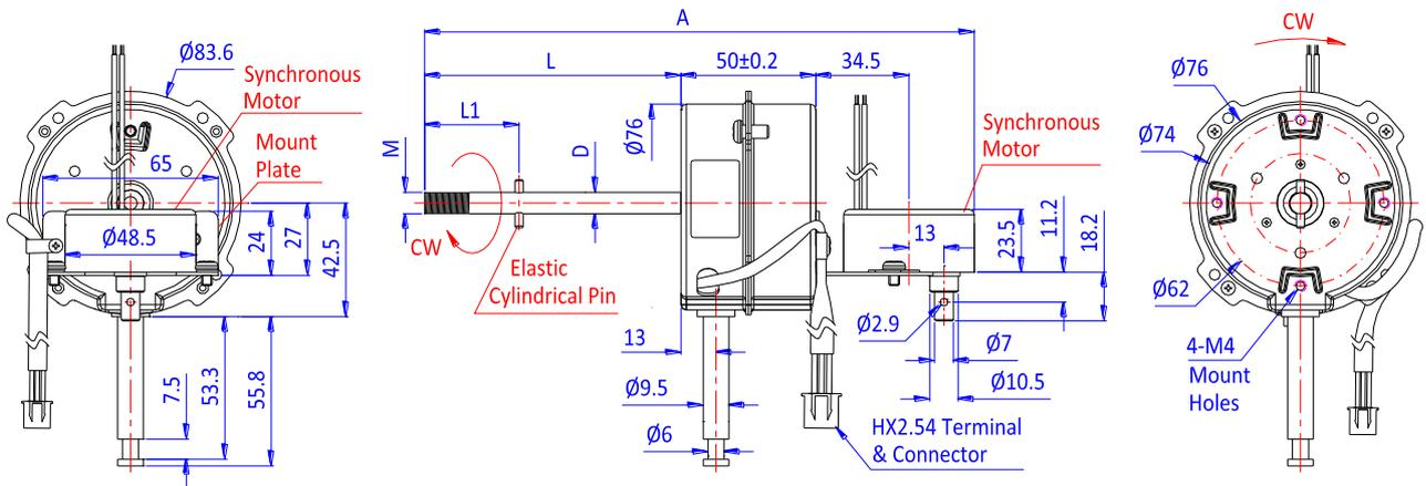
Indication of Letters: D: Shaft Diameter L: Shaft Extended Length A: Motor Body Total Length
