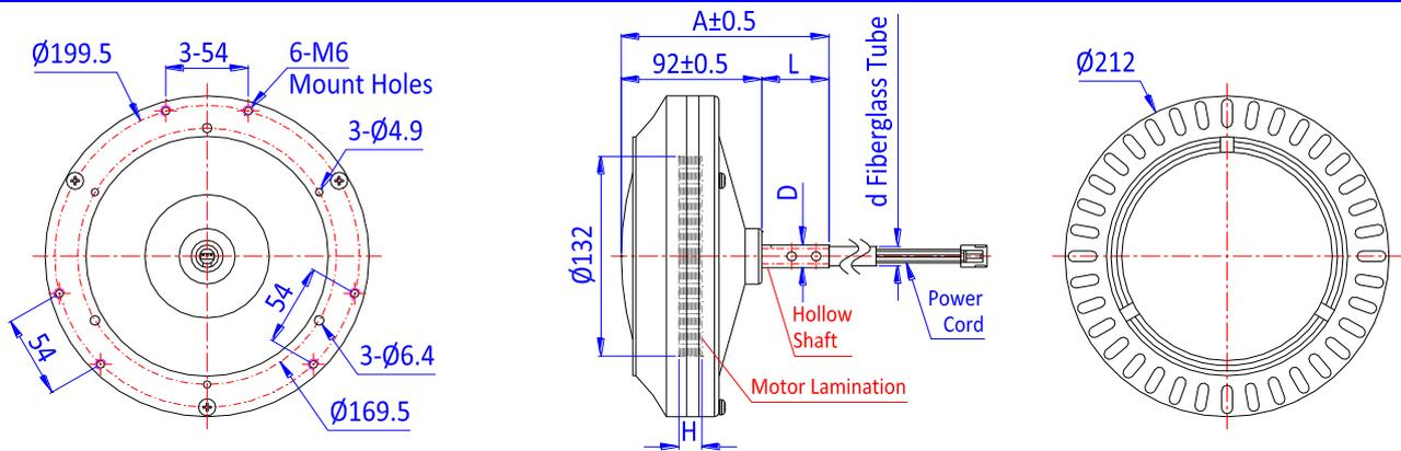
**A:** Shaft Total Length    **D:** Shaft Diameter    **H:** Lamination Height    **L:** Shaft Extended Length    **A:** Motor Total Height
